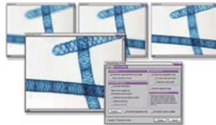
Create in-focus composite images from a series of partially in-focus images with Extended Depth of Field (EDF)
